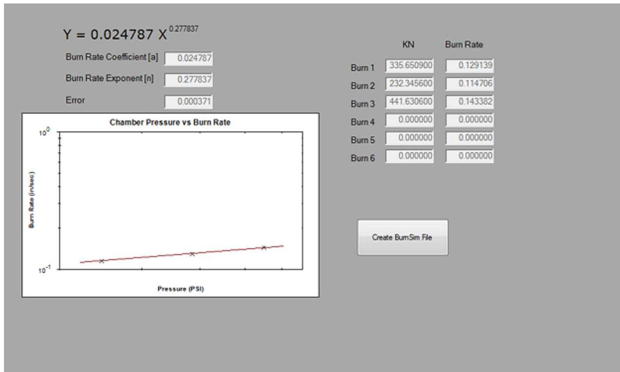
A chart is shown for Chamber Pressure vs Burn Rate. A least squares approximation line is then calculated and drawn on the graph. The a and n values are computed from the line and displayed. If the error of the line is too large (look in the ERROR Window, it should not be  $>0.009$ ) then a warning message is displayed on the screen. This probably means that one or more of the test burns is suspect and should be rerun.
